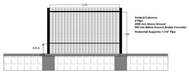
Under Ground Concrete Foundation LxWxH = 400x400x400 mm
