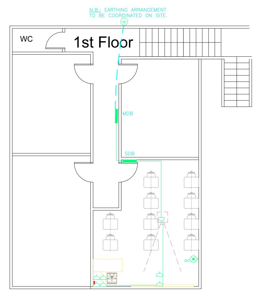
**ORGANIZATION** Right To Play Lebanon PROJECT: Ein el Helwe Center PARTNER: Naba'a **DRAWING POWER LAYOUT LEGEND** power socket earthing rod panel board ac outlet NOTES: -All installation to be exposed in pvc conduits and pvc trunks -Existing outlets to be tested. Repair/replace damaged components, if -Existing conduits can be used.
